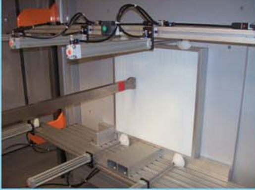
Tarama Testi (Scan Test / EN1822-4)
