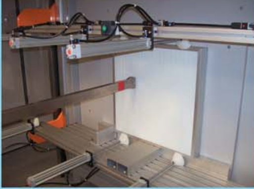
Tarama Testi (Scan Test / EN1822-4)
