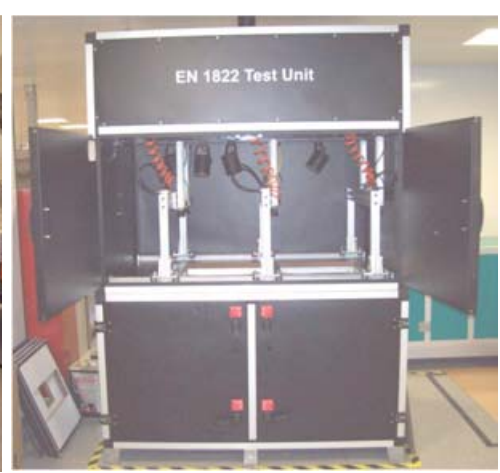
Duman testi (Oil Thread Test / EN 1822 - 4)
